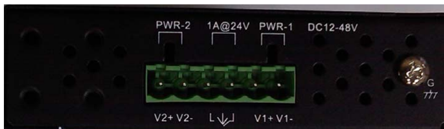
IES-2050A power connection
